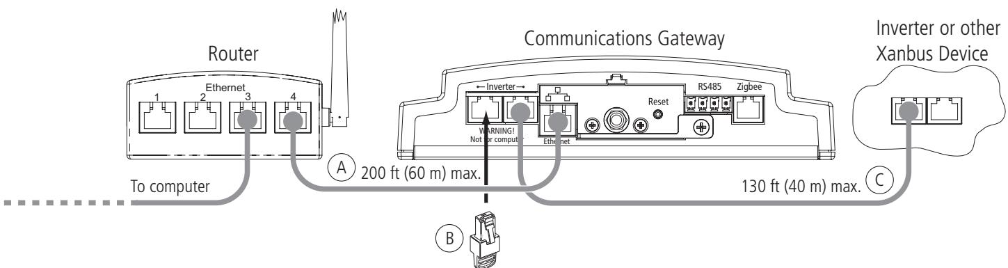
(A) Connect a cable from the Gateway Ethernet port to the router. Do not connect the Gateway to the WAN (Uplink or Internet) router port.
