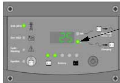
Figure 2-25 Checking Charging Operation
