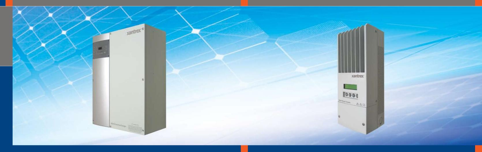
The XW Hybrid Inverter/Charger (XW) is a true sine wave inverter/charger that incorporates a DC to AC inverter, a battery charger, and an AC auto-transfer switch. It is the foundation for battery- based residential and commercial applications up to 18 kilowatts (kW). Designed for off-grid and back-up applications, the XW can operate with generators and renewable energy sources to provide full-time or backup power.
